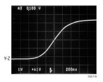
Figure 18. Driver Differential Output. R = 27  $\Omega, \ V_{CC2}$  = 5V,  $\overline{SL0}$  = 0V
