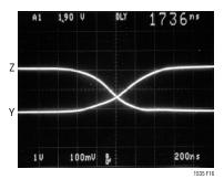
Figure 16. Driver Output. R = 27  $\Omega, V_{CC2}$  = 5V, SLO = 0V
