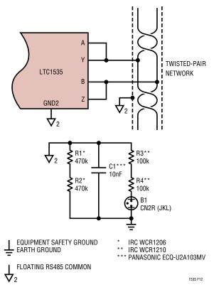
Figure 12. Detecting Fault Conditions
