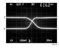
Figure 15. Driver Output. R =  $27\Omega$ , V<sub>CC2</sub> = 5V, SLO = V<sub>CC2</sub>
