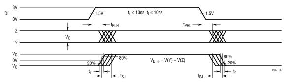
Figure 6. Driver Propagation Delays
