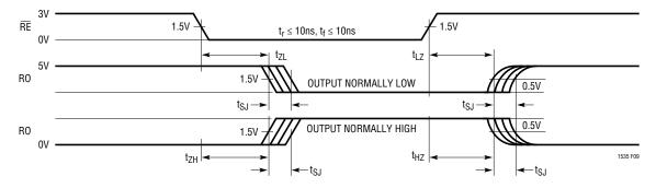
Figure 9. Receiver Enable and Disable Times
