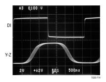
Figure 14. Driver Propagation Delay with Sample Jitter. SLO = OV
