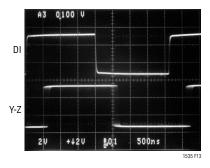
Figure 13. Driver Propagation Delay with Sample Jitter. SLO =  $V_{CC2}$
