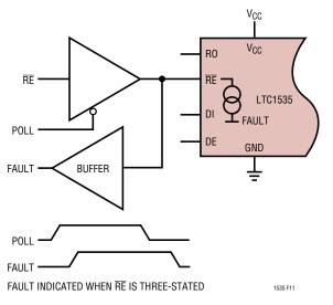
Figure 11. Detecting Fault Conditions
