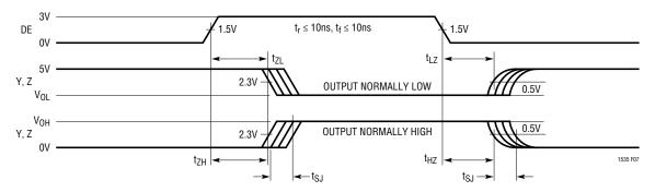
Figure 7. Driver Enable and Disable Times
