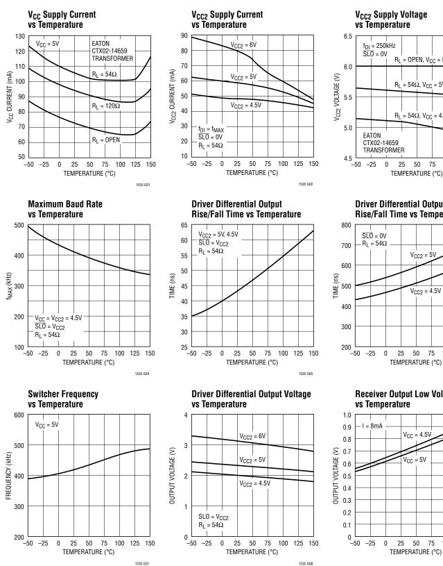
**Driver Differential Output Rise/Fall Time vs Temperature**
