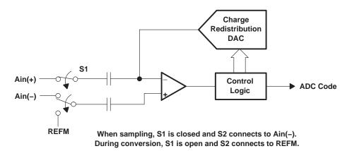
Figure 6. Simplified Pseudodifferential Input Circuit
