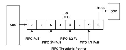
Figure 20. FIFO Structure
