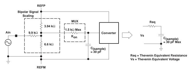
Figure 33. Equivalent Input Circuit Including the Driving Source
