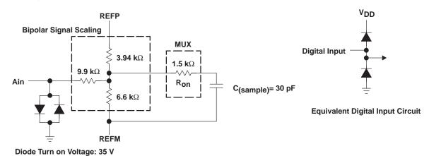
**Equivalent Analog Input Circuit**
