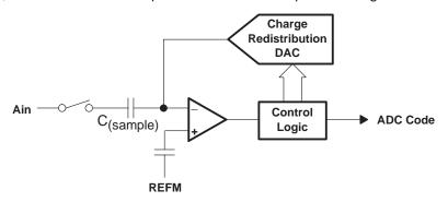
Figure 5. Simplified Block Diagram of the Successive-Approximation System
