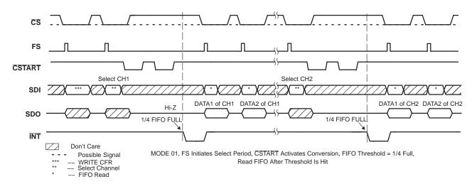
Figure 15. Mode 01, CSTART Triggers Samplings/Conversions
