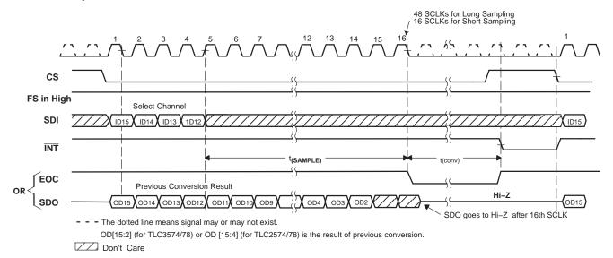
Figure 11. Mode 00, CS Initiates Operation
