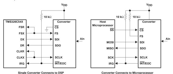
Figure 32. Typical Interface to Host DSP and Microprocessor
