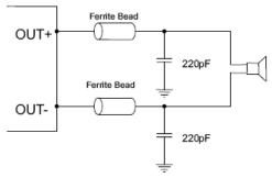
Figure 1 Ferrite Bead Filter to Reduce EMI
