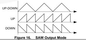
The PWM carrier frequency is decided by the PRESCAL and the POSSCAL in the SPRDH/L and SAWCNTL registers in MSFR. The PWM frequency, when SAW is in the UP-DOWN Mode, can be obtained using the following formula:
