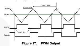
The **Sine-Wave PWM Generator** includes a Space Vector Modulation (SVM) circuit responsible for generating sine-wave PWM output waveforms. In addition to built-in sinusoidal waveform modulation, which is popular in many applications, a table allows users to customize PWM output waveforms.
