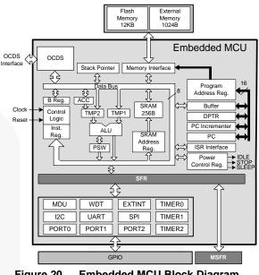
Figure 20. Embedded MCU Block Diagram
