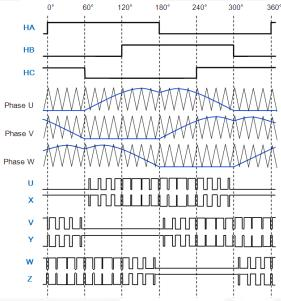
Figure 18. Default Sine-Wave PWM Output (CW=0)
