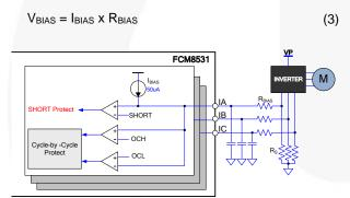
Figure 27. Current Feedback Circuit
