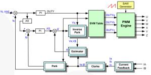
Figure 14. Sliding Mode Block Diagram
