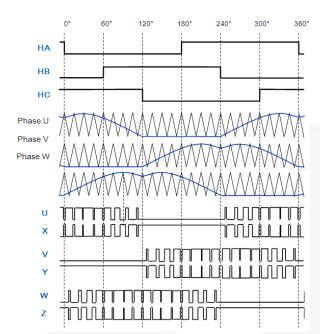
Figure 19. Default Sine-Wave PWM Output (CW=1)
