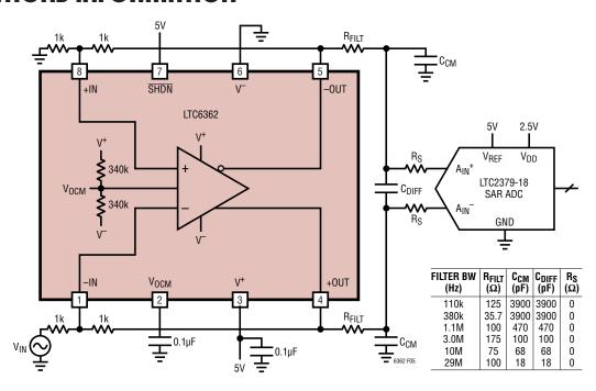
Figure 5. Recommended Interface Solutions for Driving the LTC2379-18 SAR ADC
