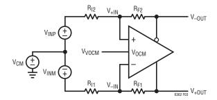
Figure 3. Real-World Application with Feedback Resistor Pair Mismatch
