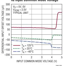
Common Mode Offset Voltage vs Temperature
