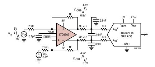
Differentially Driving an ADC with  $\Delta V_{IN} = 8V_{P-P}$  and Gain of  $A_V = 1$
