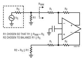
Figure 2. Optimal Compensation for Signal Source Impedance
