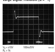
**Large-Signal Transient** (Noninverting, G = 1,  $C_L = 100pF$ )
