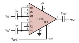
Figure 5. AC-Coupled Difference Amplifier General Configuation (G = 5 Example)
