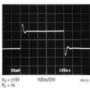
**Small-Signal Transient** (Noninverting, G = 1,  $C_L = 100pF$ )
