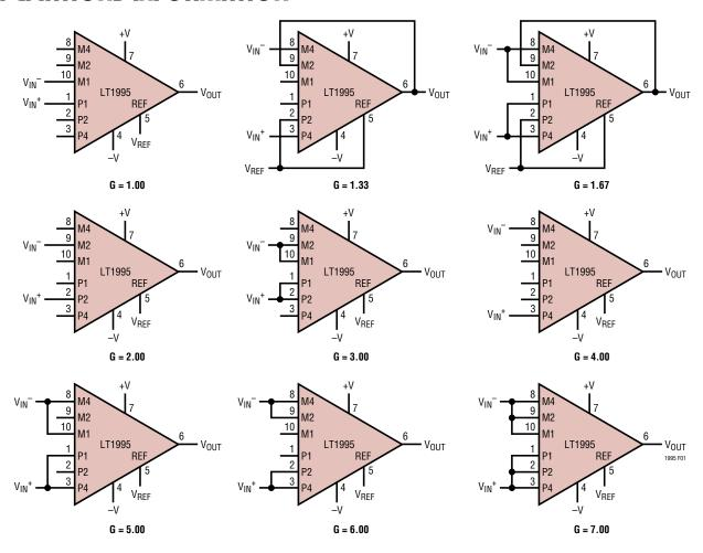
Figure 1. Difference (and Inverting) Amplifier Configurations
