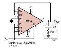
Figure 9. Optional Frequency Compensation Network for (1  $\leq$  G  $\leq$  2)
