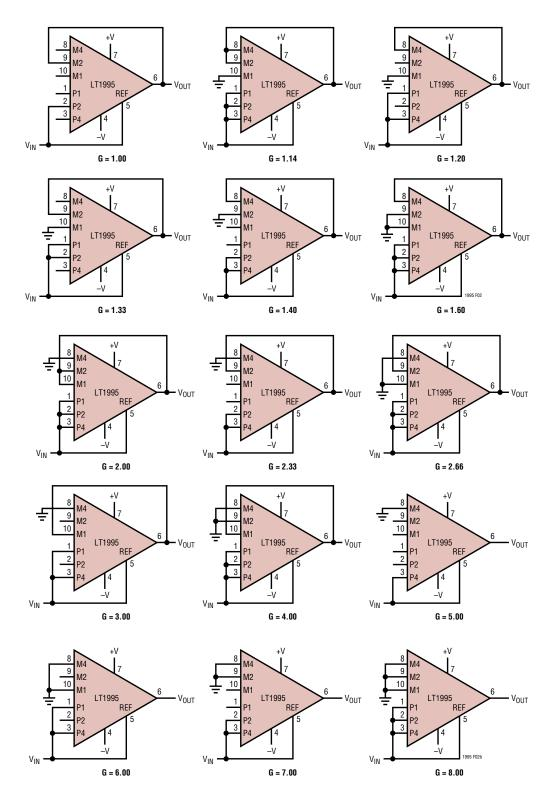
Figure 2. Noninverting Buffer Amplifier Configurations (Hi-Z Input)
