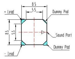
\*Unit: mm; Tolerance: ± 0.3mm Except Specified \*Housing Material: Black LCP \*Terminal plate: 3 soldering pads, tin Plating Brass
