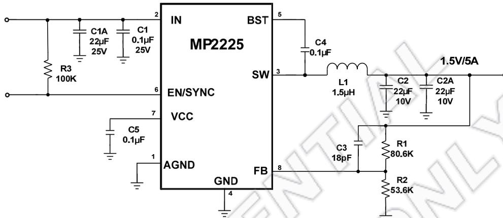
Figure 11: 12V<sub>IN</sub>, 1.5V/5A
