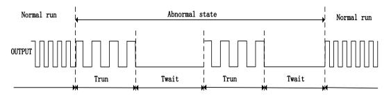
Figure 2 Lockup Protection and Automatic Restart
