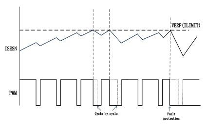
Figure 3 Cycle by cycle current protection mode
