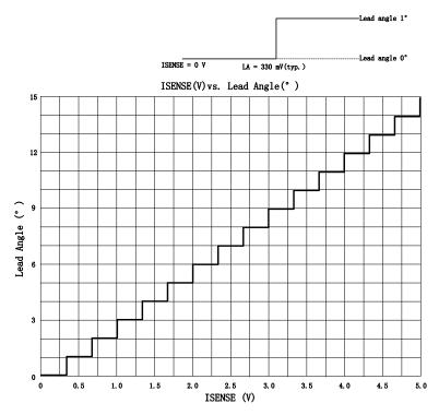
Figure 1 ISENSE vs Lead Angle
