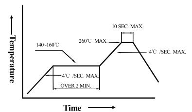
3). DIP soldering (Wave Soldering):
