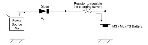
The charging voltage "Vo" must Not be higher than 3.3V (MS series) / 3.1V (ML414H) / 3.0V (TS series).
