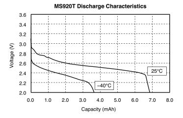
MS920T maintains about 3.5mAh at -40°C.
