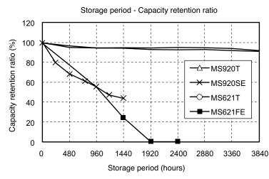
MS-T series's capacity retention ratio after High temperature storage were greatly improved.
