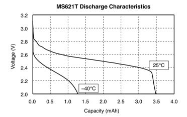
MS621T maintains about 1.2mAh at -40°C.
