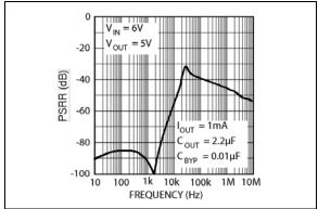
**FIGURE 2-5:** Power Supply Rejection Ratio.
