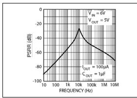
**FIGURE 2-1:** Power Supply Rejection Ratio.
