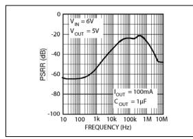
**FIGURE 2-3:** Power Supply Rejection Ratio.
