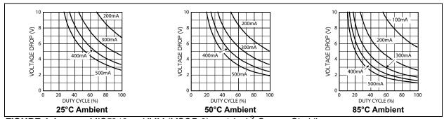
FIGURE 4-4: MIC5219-x.xYMM (MSOP-8) on 1-Inch<sup>2</sup> Copper Cladding.
