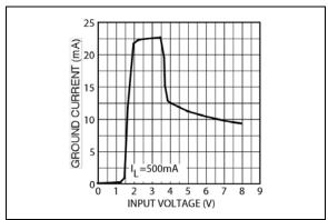
FIGURE 2-14: Ground Current vs. Supply Voltage.
