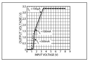
FIGURE 2-12: Dropout Characteristics.
