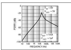
**FIGURE 2-2:** Power Supply Rejection Ratio.
