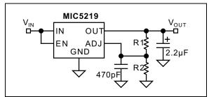
FIGURE 4-8: Ultra-Low Noise Adjustable Application.
