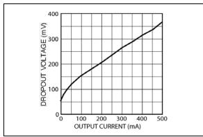
FIGURE 2-11: Dropout Voltage vs. Output Current.
