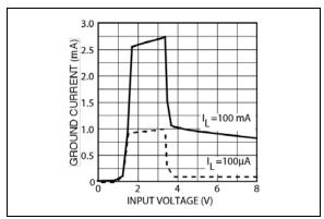
**FIGURE 2-15:** Ground Current vs. Supply Voltage.
