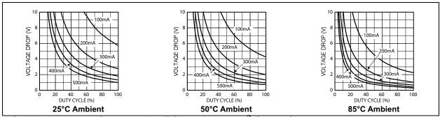
FIGURE 4-2: MIC5219-x.xYM5 (SOT23-5) on 1-Inch<sup>2</sup> Copper Cladding.
