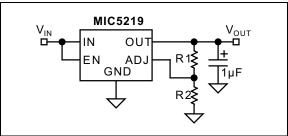
FIGURE 4-7: Low-Noise Adjustable Voltage Regulator.
