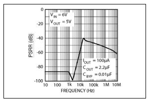
**FIGURE 2-4:** Power Supply Rejection Ratio.
