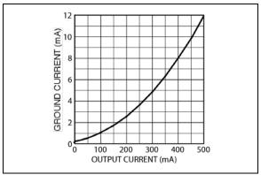
**FIGURE 2-13:** Ground Current vs. Output Current.
