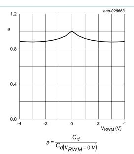
Fig. 4. Relative capacitance as a function of reverse standoff voltage; typical values
