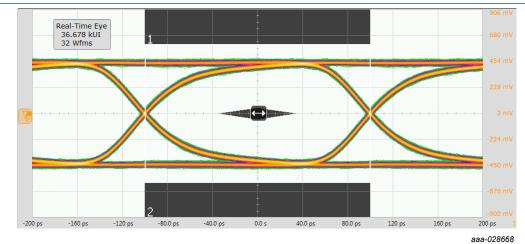
Fig. 9. USB 3.2 eye diagram, PCB without device; typical values
