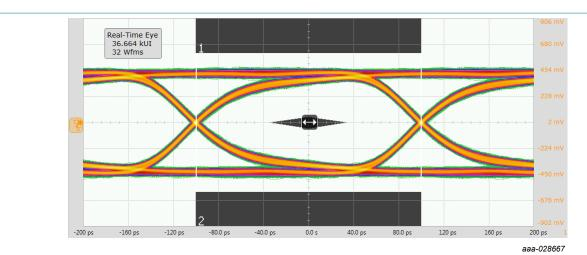
Fig. 8. USB 3.2 eye diagram, PCB with device; typical values
