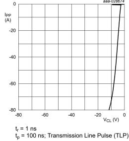
Fig. 15. Dynamic resistance with negative clamping;
