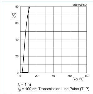
Fig. 14. Dynamic resistance with positive clamping; typical values
