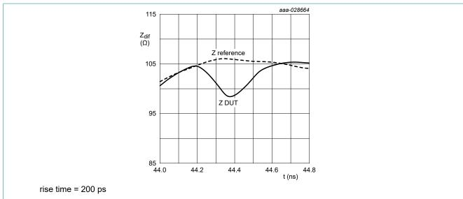
Fig. 5. Differential Time Domain Reflectometer (TDR) plot; typical values
