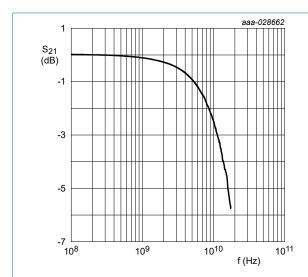
Fig. 3. Insertion loss; typical values
