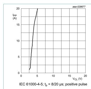
Fig. 18. Dynamic resistance with positive clamping; typical values
