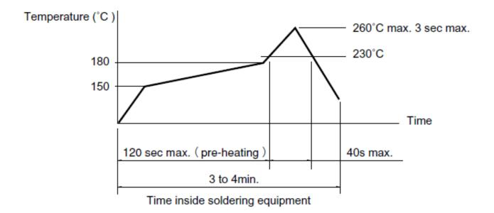
(1) The above temperature shall be measured of the top of switch. There are cases where PC board's temperature greatly differs from that of the switch, depending on the material, size, thickness of PC board's and others. Care, should be taken to prevent the switch's surface temperature from exceeding  $260^{\circ}$ C.
