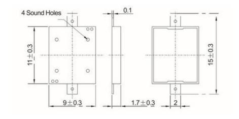
\*Unit: mm; Tolerance: ± 0.3mm Except Specified
