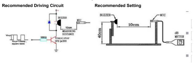
Resonant frequency, 1/2 duty cycle. Square wave. Signal amplitude should be large enough tosaturate the transistor.
