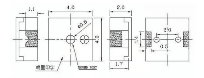
\*Unit: mm; Tolerance: ± 0.3mm Except Specified
