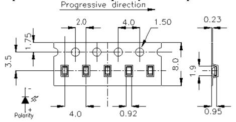
**Note:** The tolerances unless mentioned are  $\pm 0.1$ mm, unit = mm
