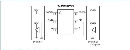
Fig 9. Unidirectional logic level-shifting application
