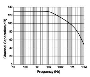
Channel Separation as a function of Frequency.
