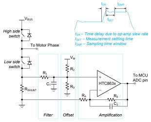
Figure 8. Current Shunt Monitor Circuit
