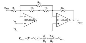
Figure 6. Instrumentation Amplifier
