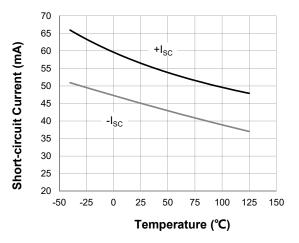
Short-circuit Current as a function of Temperature.
