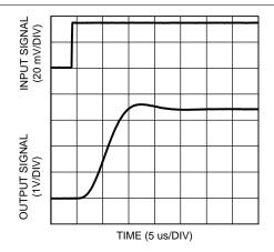
Figure 30. Settling Time (Rising Edge) at  $V_S = 5 \text{ V}$ LMP8603 and LMP8603-Q1
