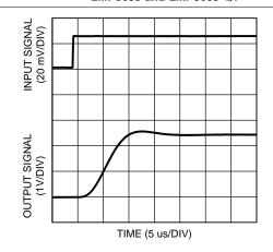
Figure 29. Settling Time (Rising Edge) at V<sub>S</sub> = 3.3 V LMP8603 and LMP8603-Q1
