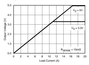
Figure 61. Expected Output Voltage vs Load Current Using 15-mΩ Sense Resistor
