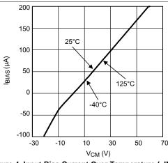
Figure 4. Input Bias Current Over Temperature (+IN and -IN pins) at V<sub>S</sub> = 5 V
