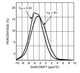
Figure 39. Gain Drift Distribution, 5000 Parts LMP8602 and LMP8602-Q1
