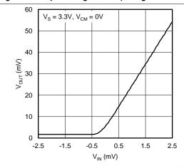
Figure 52. Output Voltage vs VIN (Enlarged Close to 0 V)
