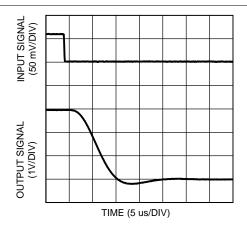
Figure 22. Settling Time (Falling Edge) at V<sub>S</sub> = 5 V LMP8602 and LMP8602-Q1
