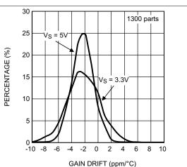
Figure 38. Gain Drift Distribution, 1300 Parts LMP8601 and LMP8601-Q1
