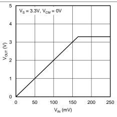
Figure 51. Output Voltage vs VIN
