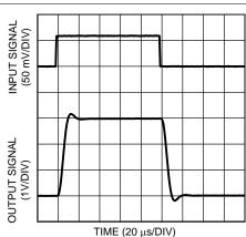
Figure 20. Step Response at  $V_S = 5$  V,  $R_L = 10$  k $\Omega$  LMP8602 and LMP8602-Q1
