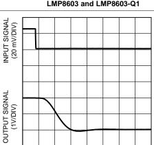
Figure 27. Settling Time (Falling Edge) at V<sub>S</sub> = 3.3 V LMP8603 and LMP8603-Q1
