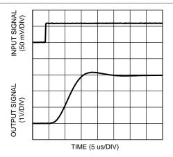
Figure 24. Settling Time (Rising Edge) at V<sub>S</sub> = 5 V LMP8602 and LMP8602-Q1
