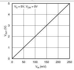
Figure 49. Output Voltage vs VIN
