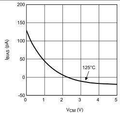
Figure 5. Input Bias Current Over Temperature (A2 pin) at  $\rm V_S = 5~\rm V$
