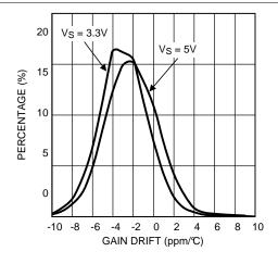
Figure 46. Gain Error Distribution at V<sub>S</sub> = 5 V LMP8603 and LMP8603-Q1
