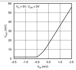
Figure 50. Output Voltage vs VIN (Enlarged Close to 0 V)
