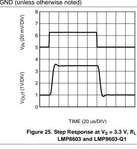
Figure 25. Step Response at  $V_S$  = 3.3 V,  $R_L$  = 10 k $\Omega$
