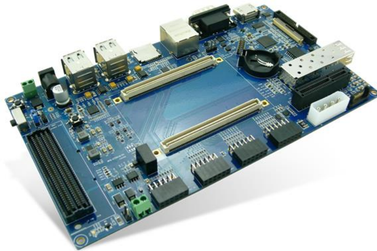
Figure 1-6 MYD-C7Z015 Base Board for MYC-C7Z015 CPU Module
