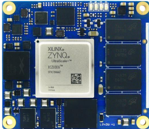
Figure 1-6 MYC-CZU3EG CPU Module Top-view
