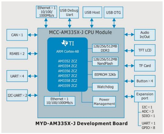
Figure 1-6 Function Block Diagram of MYD-AM335X-J
