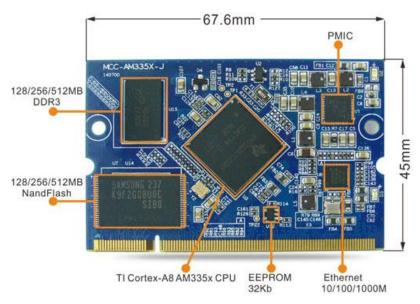
Figure 1-3 MCC-AM335X-J CPU Module
