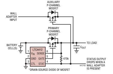
Figure 2. Automatic Switchover of Load Between a Battery and a Wall Adapter with Auxiliary P-Channel MOSFET for Lowest Loss
