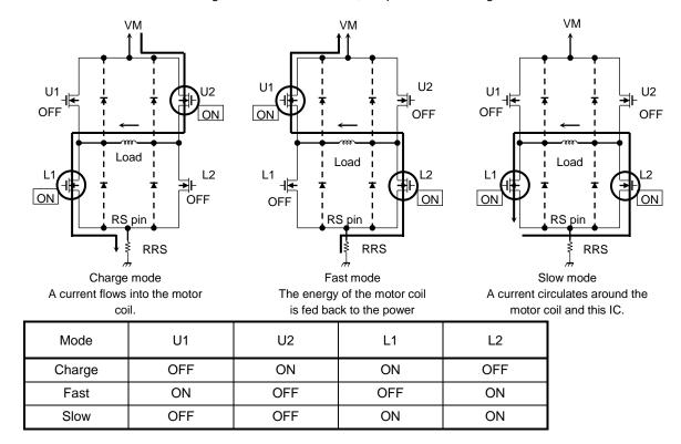
This IC controls the motor current to be constant by 3 modes listed above.
