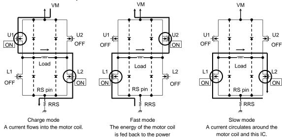
**Operation Function of Output Transistor**
