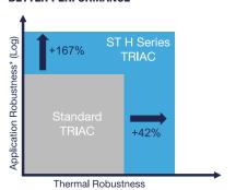
\*Application robustness includes noise immunity (dV/dt) and turn-off commutation (dl/dt) $_{\rm c}$  under resistive and inductive loads
