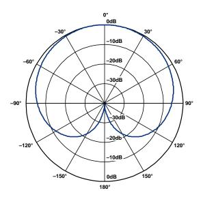
Figure 9. Response of a 2-Microphone Endfire Cardioid Beamformer
