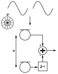
Figure 8. 2-Microphone Endfire Array
