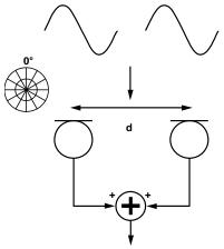
Figure 3. 2-Microphone Broadside Array
