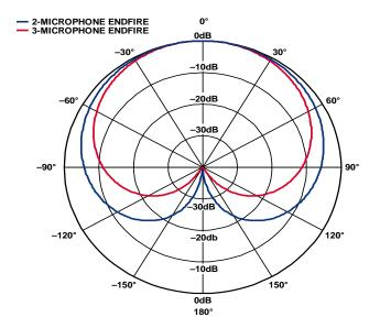
Figure 14. Comparison of First-Order and Second-Order Endfire Beamformers
