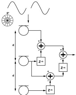
Figure 13. Second-Order Differential Beamforming Array
