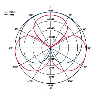
Figure 10. Frequency Aliasing in a 2-Microphone Endfire Beamformer
