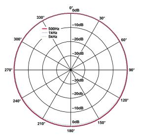
Figure 2. Omnidirectional Microphone Response Plot
