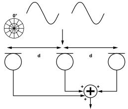
Figure 6. 3-Microphone Broadside Array
