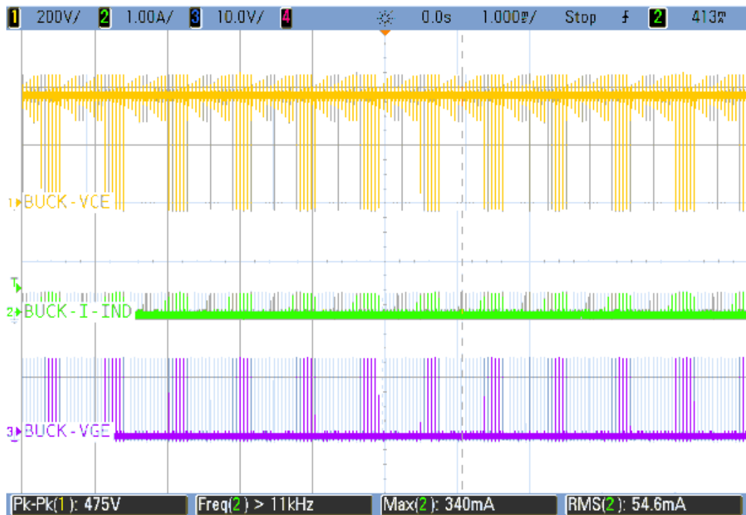
Figure 53. Buck converter - Analog dimming - V_{CE} vs I_{INDUCTOR} vs V_{GE} at 0.5%
