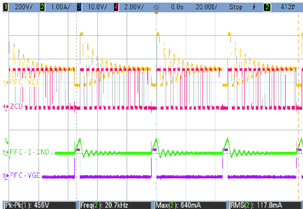
Figure 33. PFC working in Discontinuous Mode V_{CE} vs ZCD vs I_{\text{Inductor}} vs V_{GE} at 110 V AC
