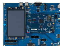
STM32MP157A-EV1 STM32MP157C-EV1 2 Evaluation boards
