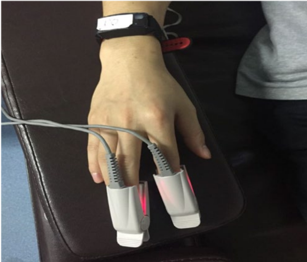
Figure 7. Maxim's sensor placed in a wrist watch. The finger clips of two reference devices are attached to the index and middle fingers of the test subject
