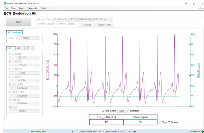
Figure 4. Evaluation Software Analyzes ECG Measurements
