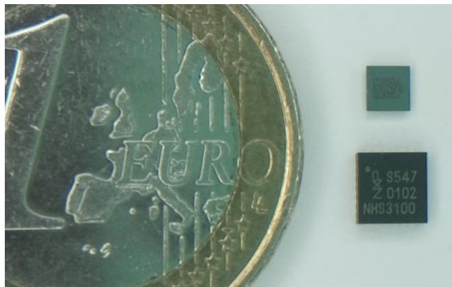
Figure 1: €1 and two NHS3xxx in a CSP and HVQfn24 package
