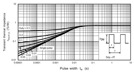
Fig. 8.13 r<sub>th</sub> - t<sub>w</sub> (Guaranteed Maximum)
