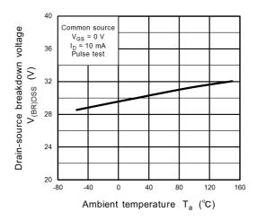
Fig. 8.7 V<sub>(BR)DSS</sub> - T<sub>a</sub>
