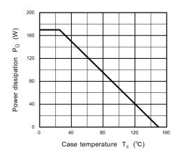
$\label{eq:Fig. 8.15} \begin{array}{ll} Fig.~8.15 & P_D - T_C \\ \text{(Guaranteed Maximum)} \end{array}$
