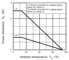
Fig. 8.14 P<sub>D</sub> - T<sub>a</sub> (Guaranteed Maximum)
