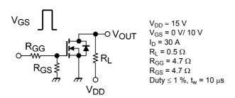
Fig. 6.2.1 Switching Time Test Circuit
