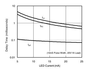
Figure 7. Typical Delay Times
