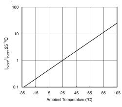
Figure 5. Typical Normalized Off-State Leakage
