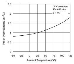
Figure 4. Typical Normalized On-Resistance
