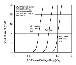
Figure 6. Input Characteristics (Current Controlled)
