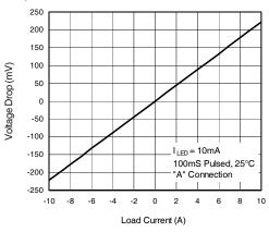
Figure 3. Linearity Characteristics
