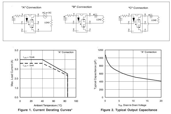
\* Derating of 'B' and 'C' connections at +85°C will be 70% of that specified at +40°C and is linear from +40°C to +85°C.
