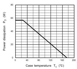
Fig. 8.15 P<sub>D</sub> - T<sub>c</sub> (Guaranteed Maximum)
