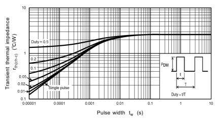
Fig. 8.13 r<sub>th</sub> - t<sub>w</sub> (Guaranteed Maximum)
