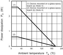
Fig. 8.14 P<sub>D</sub> - T<sub>a</sub> (Guaranteed Maximum)
