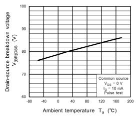
Fig. 8.7 V<sub>(BR)DSS</sub> - T<sub>a</sub>
