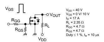
Fig. 6.2.1 Switching Time Test Circuit
