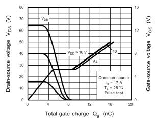
Fig. 8.10 Dynamic Input/Output Characteristics
