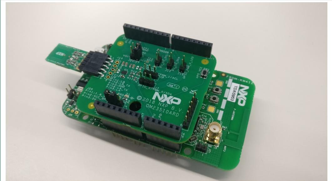
Figure 3. Connection between FRDM-KW41Z board and OM2NTx5332
