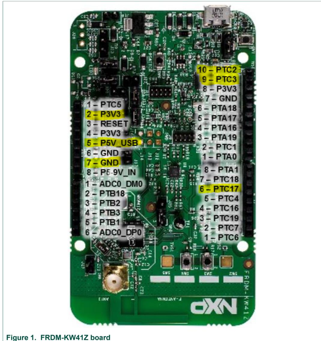
Figure 1. FRDM-KW41Z board
