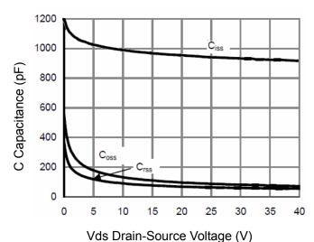
Figure 11 Capacitance vs Vds
