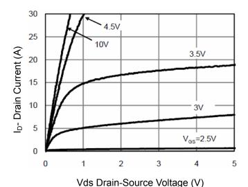
**Figure 3 Output Characteristics**
