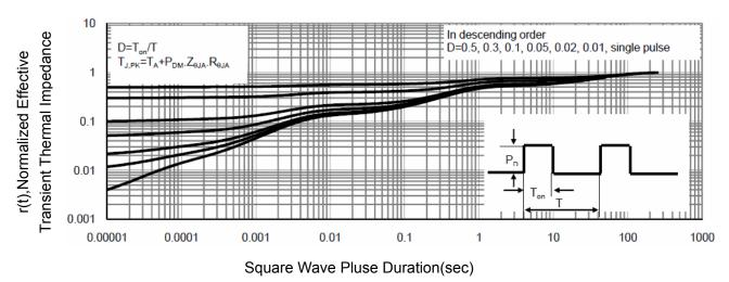
**Figure 13 Normalized Maximum Transient Thermal Impedance**
