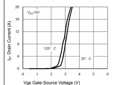
**Figure 4 Transfer Characteristics**
