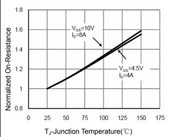
Figure 6 Drain-Source On-Resistance
