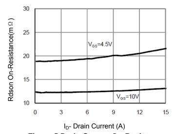
Figure 5 Drain-Source On-Resistance
