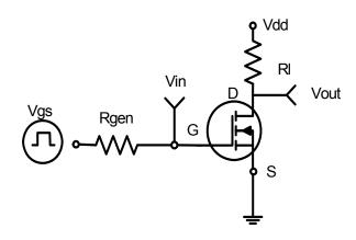
**Figure 1:Switching Test Circuit**
