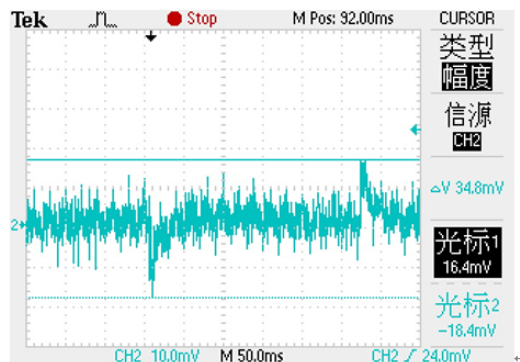
15. Load transient response (IL=10-350-10mA)
