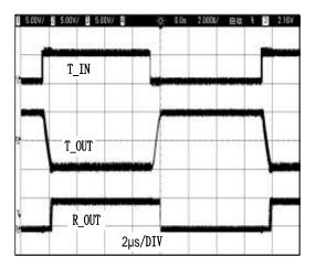
Figure 5. Loopback Test At 333kbps
