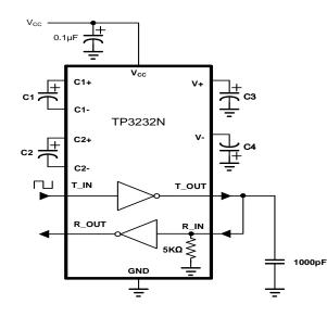
Figure 4. Loopback Test Circuit
