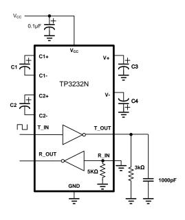
Figure 1. Slew-Rate Test Circuits
