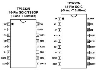
Microamp Supply-Current, 3.0V to 5.5V, Up to 470kbps RS-232 Transceivers
