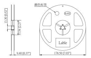
Dimensions of Tape (Unit: mm)
