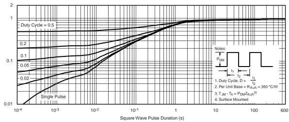
Normalized Thermal Transient Impedance, Junction-to-Ambient
