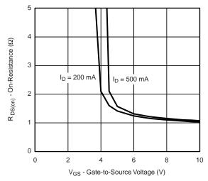
On-Resistance vs. Gate-Source Voltage
