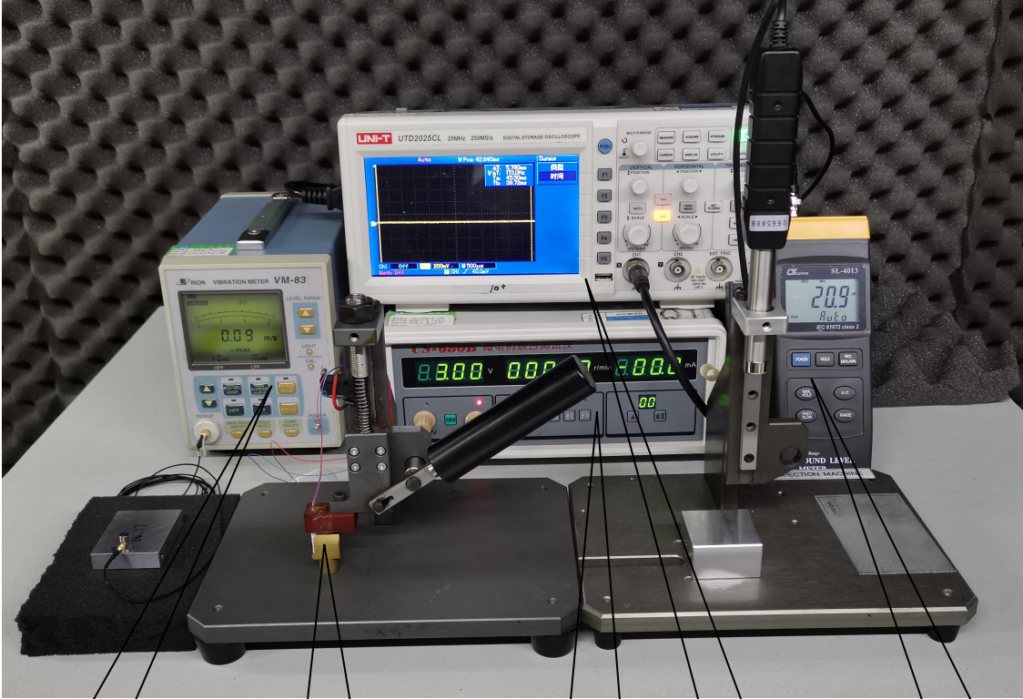
马达安放装置 Test Jig (for Clamping the Motor in Place)
