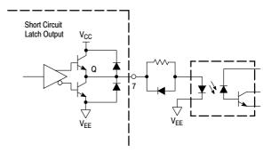
Figure 33. Output Fault Optoisolator
