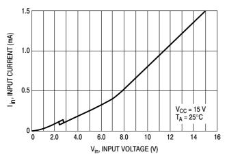
Figure 2. Input Current versus Input Voltage
