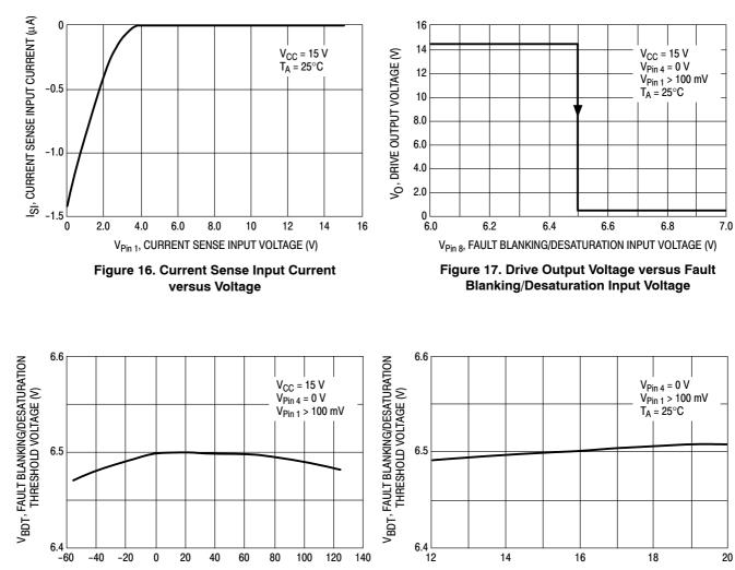
Figure 18. Fault Blanking/Desaturation Comparator Threshold Voltage versus Temperature
