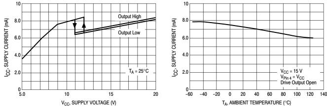
Figure 28. Supply Current versus Supply Voltage
