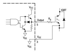
Figure 31. Using a Single Gate Resistor
