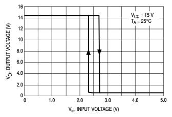
Figure 3. Output Voltage versus Input Voltage
