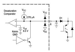
Figure 34. Desaturation Detection
