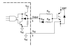
Figure 32. Using Separate Resistors for Turn-On and Turn-Off
