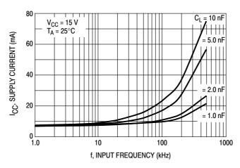
Figure 30. Supply Current versus Input Frequency
