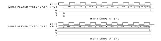
Figure 4-16: H:V:F Output Timing - HD 10-bit Output Mode
