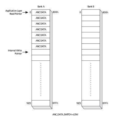
Figure 4-32: Ancillary Data Extraction - Step A
