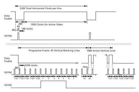
Figure 4-25: H:V:DE Output Timing 1920 x 1080p @ 59.94/60 (Format 16)
