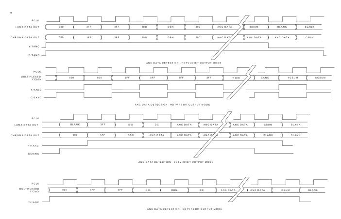
Figure 4-31: Y/1ANC and C/2ANC Signal Timing
