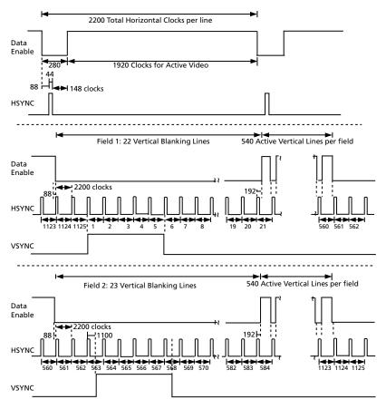
Figure 4-20: H:V:DE Output Timing 1920 x 1080i @ 59.94/60 (Format 5)
