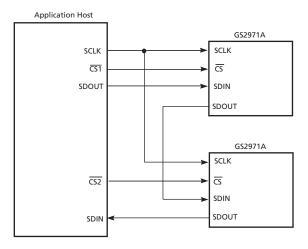
Figure 4-48: GSPI Application Interface Connection
