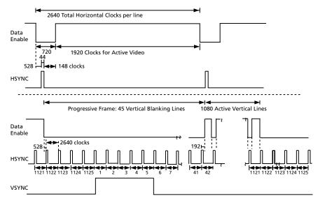
Figure 4-28: H:V:DE Output Timing 1920 x 1080p @ 25 (Format 33)
