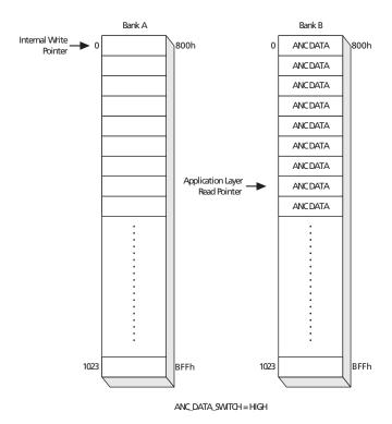
Figure 4-35: Ancillary Data Extraction - Step D
