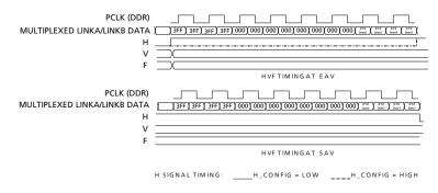
Figure 4-14: H:V:F Output Timing - 3G Level B 10-bit Mode
