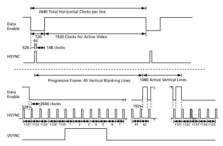
Figure 4-26: H:V:DE Output Timing 1920 x 1080p @ 50 (Format 31)
