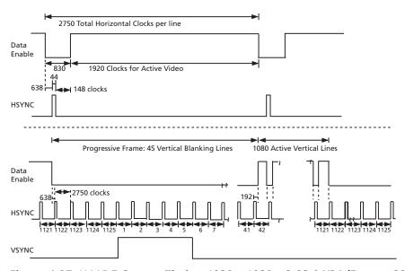
Figure 4-27: H:V:DE Output Timing 1920 x 1080p @ 23.94/24 (Format 32)
