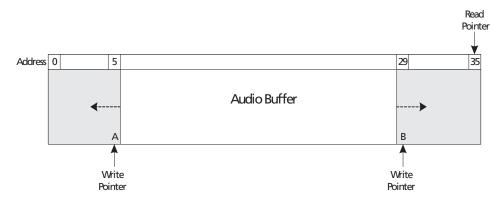
Figure 4-47: Audio Buffer Pointer Boundary Checking
