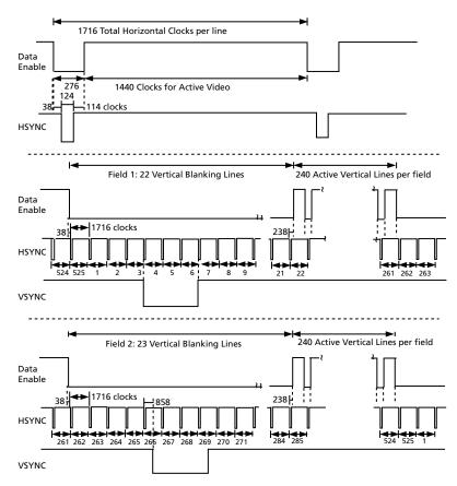
Figure 4-21: H:V:DE Output Timing 720 (1440) x 480i @ 59.94/60 (Format 6&7)
