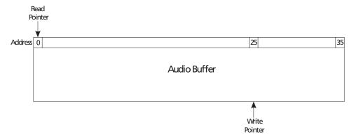
Figure 4-46: Audio Buffer After Initial 26 Sample Write
