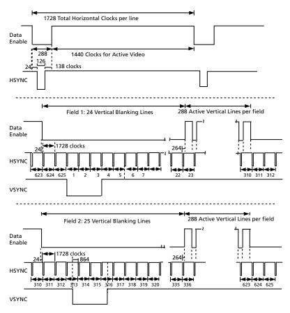
Figure 4-24: H:V:DE Output Timing 720 (1440) x 576 @ 50 (Format 21 & 22)
