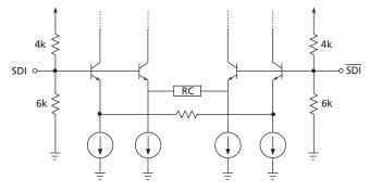
Figure 3-9: Equalizer Input Equivalent Circuit
