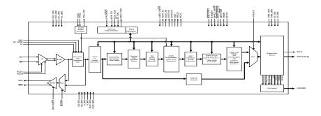
Figure 4-3: GS2971A Integrated EQ Block Diagram
