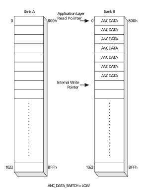
Figure 4-34: Ancillary Data Extraction - Step C
