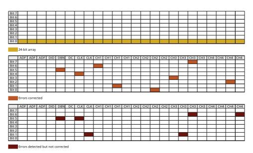
Figure 4-44: ECC 24-bit Array and Examples
