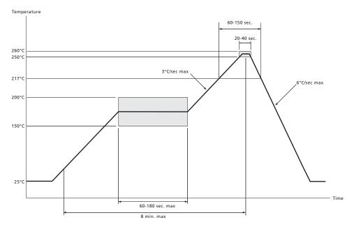
Figure 7-3: Pb-free Solder Reflow Profile
