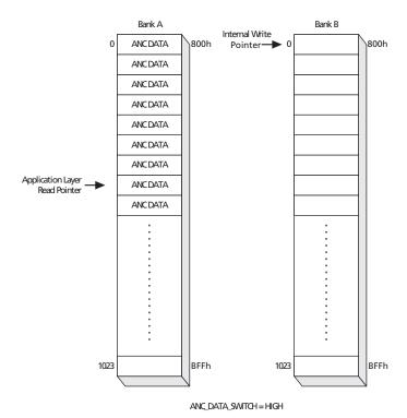
Figure 4-33: Ancillary Data Extraction - Step B
