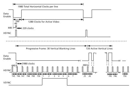
Figure 4-22: H:V:DE Output Timing 1280 x 720p @ 50 (Format 19)
