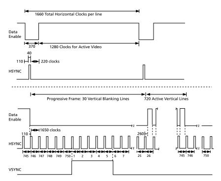
Figure 4-19: H:V:DE Output Timing 1280 x 720p @ 59.94/60 (Format 4)
