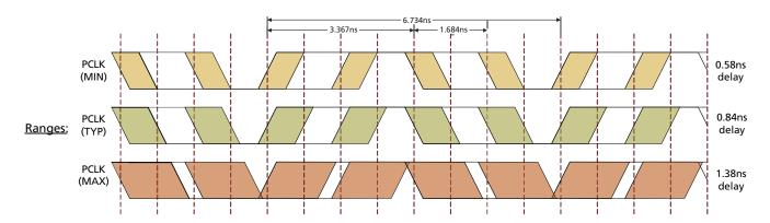
Figure 4-10: Delay Adjustment Ranges
