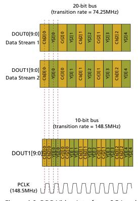
Figure 4-9: DDR Video Interface - 3G Level B
