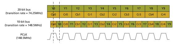
Figure 4-8: DDR Video Interface - 3G Level A
