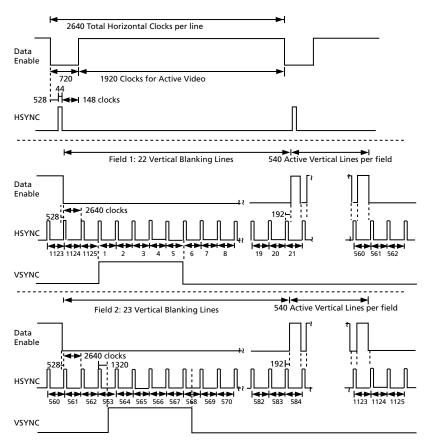
Figure 4-23: H:V:DE Output Timing 1920 x 1080i @ 50 (Format 20)
