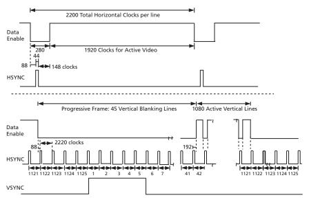
Figure 4-29: H:V:DE Output Timing 1920 x 1080p @ 29.97/30 (Format 34)
