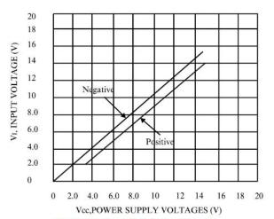
Figure 1.Input Voltage Range
