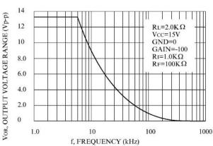
Figure 3. Large-Signal Frequency Response
