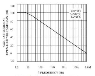
Figure 2. Open-Loop Frequency
