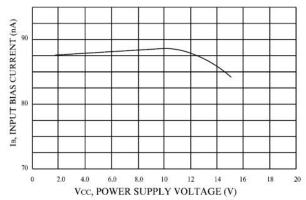
Figure 6. Input Bias Current versus Power Supply Voltage
