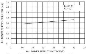
Figure 5. Power Supply Current versus Power Supply Voltage
