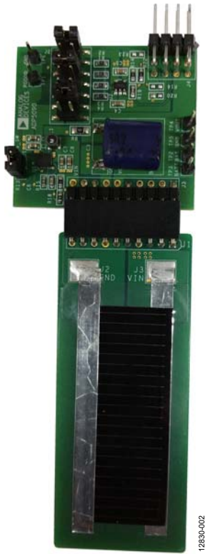
Figure 2. ADP5090-2-EVALZ Board Hardware
