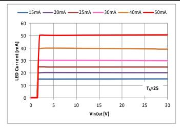
Figure 14 LED Current vs. VInOut
