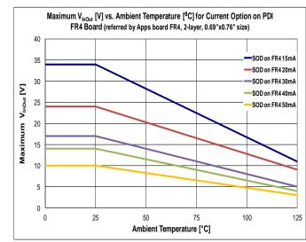
Figure 11 Maximum VInOut vs. Temperature
