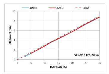
Figure 5 PWM Dimming 30mA vs. Duty Cycle
