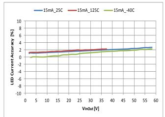
Figure 17 LED Current Accuracy (%) vs. VInOut across Temperature
