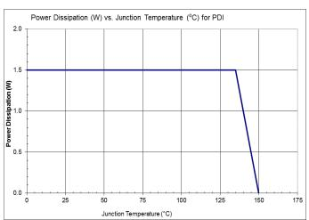
Figure 13 Power Dissipation vs. Junction Temperature
