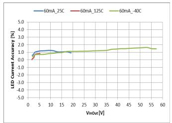
Figure 23 LED Current Accuracy (%) vs. VInOut across Temperature
