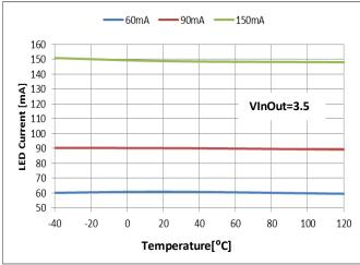
Figure 22 LED Current across Temperature
