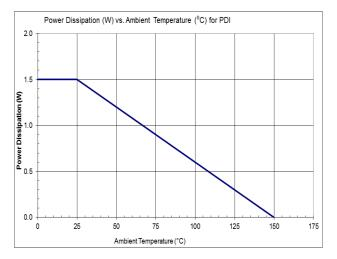
Figure 12 Power Dissipation vs. Ambient Temperature
