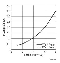
Figure 8.  $5V_{\text{IN}},$  3.3V and 1.5V\_{\text{OUT}} Power Loss
