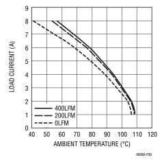
Figure 9. No Heat Sink with  $3.3V_{\text{IN}}$  to  $1.5V_{\text{OUT}}$
