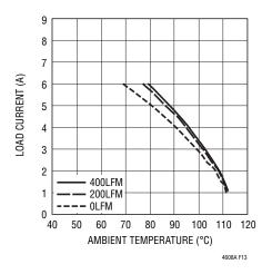
Figure 13. No Heat Sink with  $\rm 3.3V_{IN}$  to  $\rm 2.5V_{OUT}$
