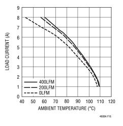
Figure 16. BGA Heat Sink with  $5V_{\text{IN}}$  to  $3.3V_{\text{OUT}}$
