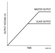
Figure 6. Output Voltage Coincident Tracking
