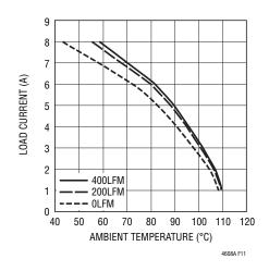
Figure 11. No Heat Sink with  $5V_{\text{IN}}$  to  $1.5V_{\text{OUT}}$
