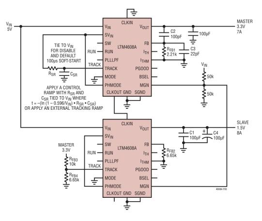
Figure 5. Dual Outputs (3.3V and 1.5V) with Tracking
