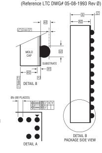
$\begin{array}{c} \text{BGA Package} \\ \text{68-Lead} \ (15.00 \text{mm} \times 9.00 \text{mm} \times 3.42 \text{mm}) \end{array}$
