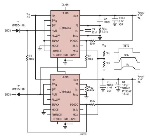
Figure 20. Dual LTM4608A Output Sequencing Application. See Also Dual 8A per Channel LTM4616
