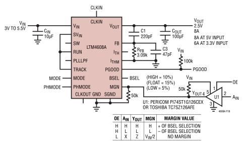
Figure 18. Typical 3V to  $5.5V_{IN}$ , 2.5V at 8A Design
