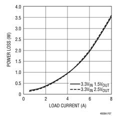
Figure 7. 3.3  $V_{\text{IN}},$  2.5 V and 1.5  $V_{\text{OUT}}$  Power Loss
