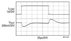
1A TO 3A TRANSIENT 12V<sub>IN</sub> TO  $5V_{OUT}$  C<sub>OUT</sub> =  $2\times47\mu$ F FRONT PAGE APP
