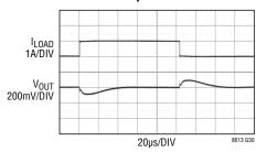
1A TO 2A TRANSIENT 12V<sub>IN</sub> TO  $5V_{OUT}$  C<sub>OUT</sub> =  $2\times47\mu$ F FRONT PAGE APP
