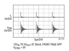
Figure 2. Burst Mode Operation
