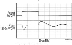
0.1A TO 1.1A TRANSIENT 12V<sub>IN</sub> TO 5V<sub>OUT</sub> C<sub>OUT</sub> = 2×47µF FRONT PAGE APP
