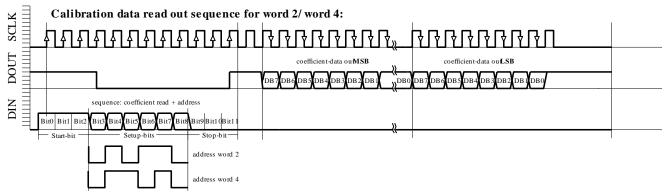
Fig. 6d: W2, W4 READING sequence
