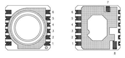
Fig. 2: Pin configuration of MS5535C
