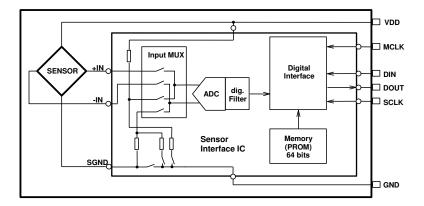
Fig. 1: Block diagram MS5535C
