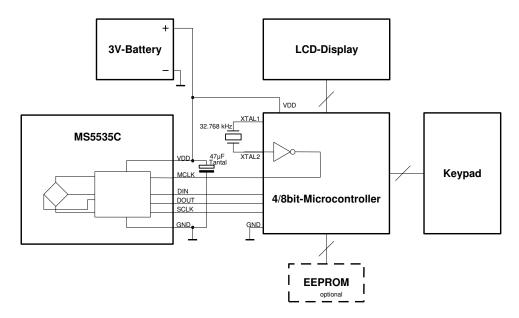
Figure 7: Demonstration of MS5535C in a diving computer.
