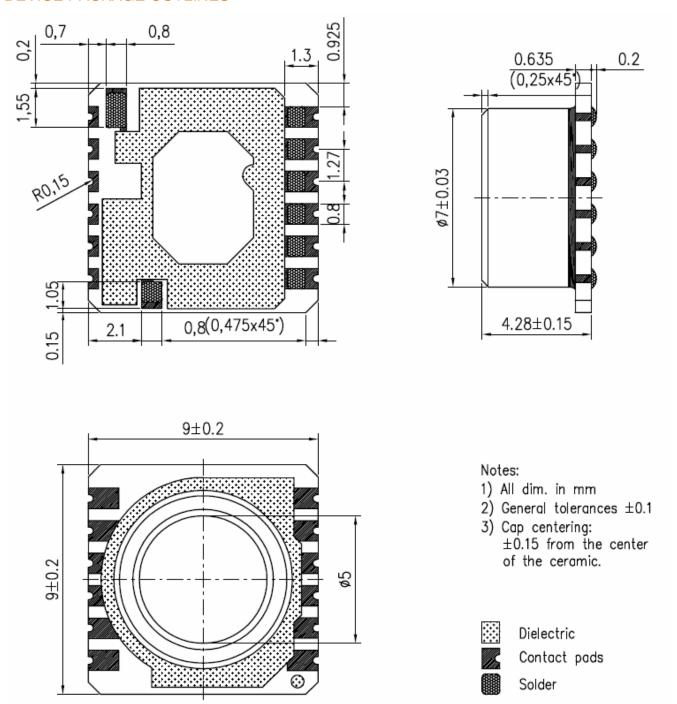
Fig. 8: Device package outlines of MS5535-CM
