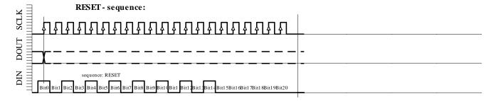
Fig. 6e: RESET sequence (21 bit)
